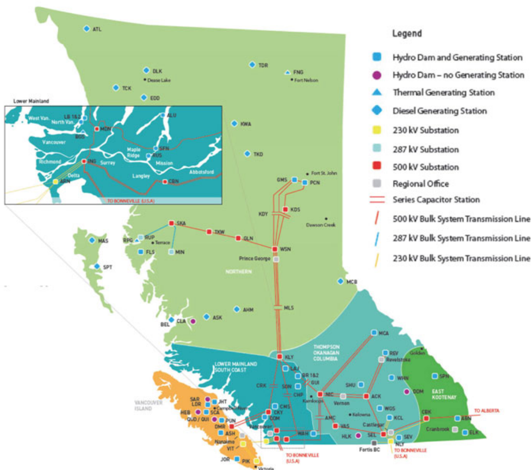
Figure 2. Diesel generators are mostly found in the remote north of the province and generally do not occur near major transmission infrastructure 14 .
